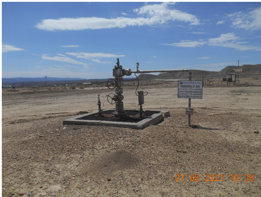
Injection wellhead
