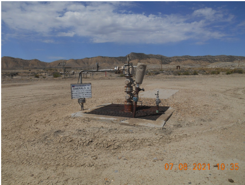
Injection wellhead
