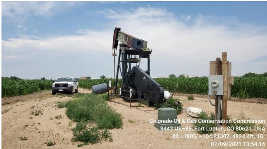
**Photo 5 pump jack, meter box, electric panel and transformers**
