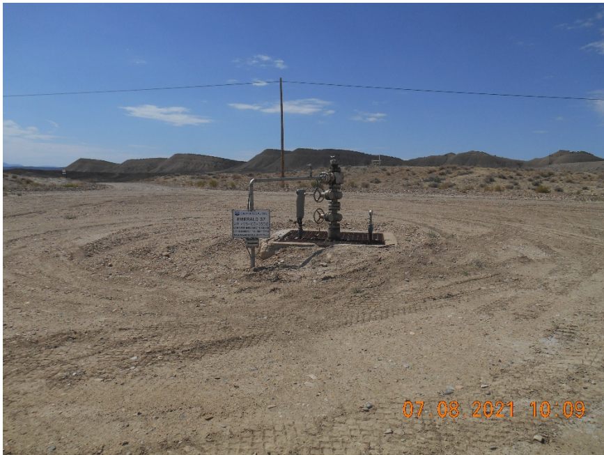
Injection wellhead.
