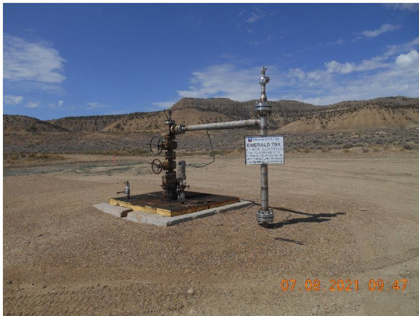
Injection wellhead
