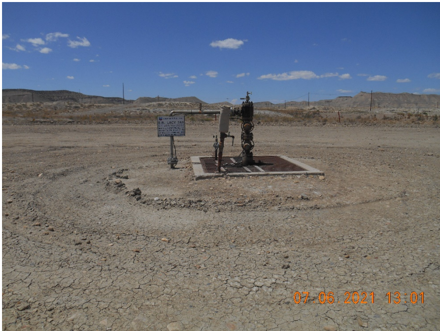
Injection wellhead.
