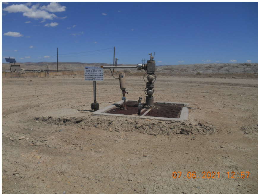
Injection wellhead
