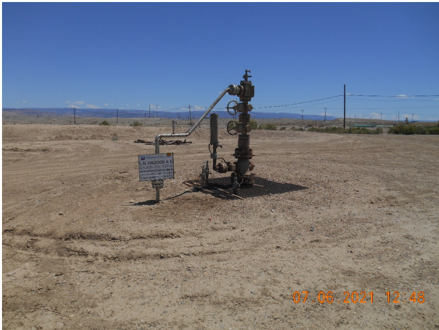
Injection wellhead.
