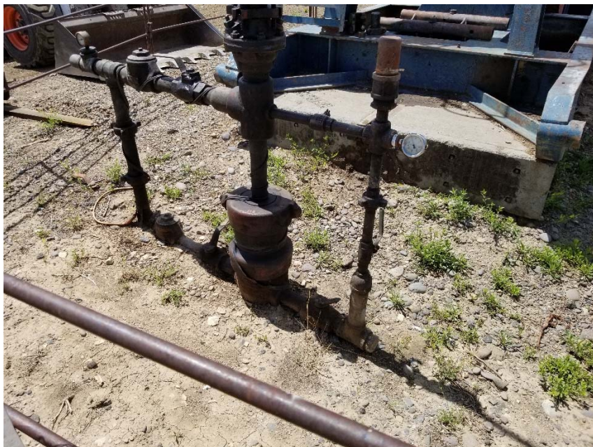
Photo 2. No bradenhead access apparent.
