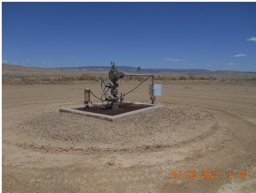
Injection wellhead
