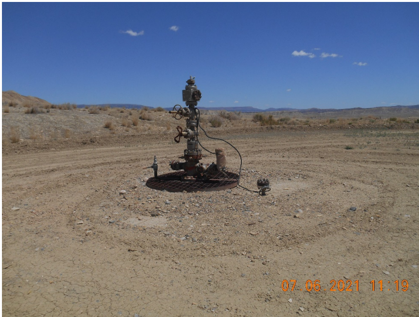
Injection wellhead
