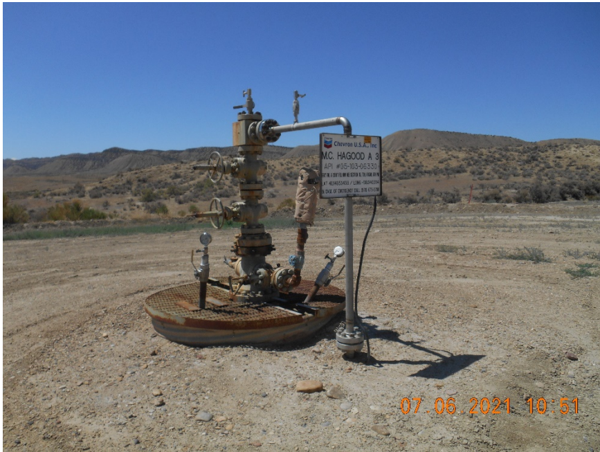
Injection wellhead
