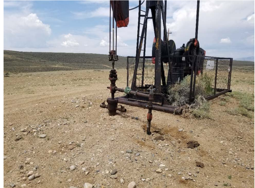
Photo 2. No bradenhead access apparent.
