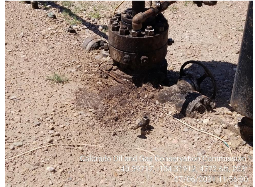
Photo 10 – Stained Soil at Wellhead
