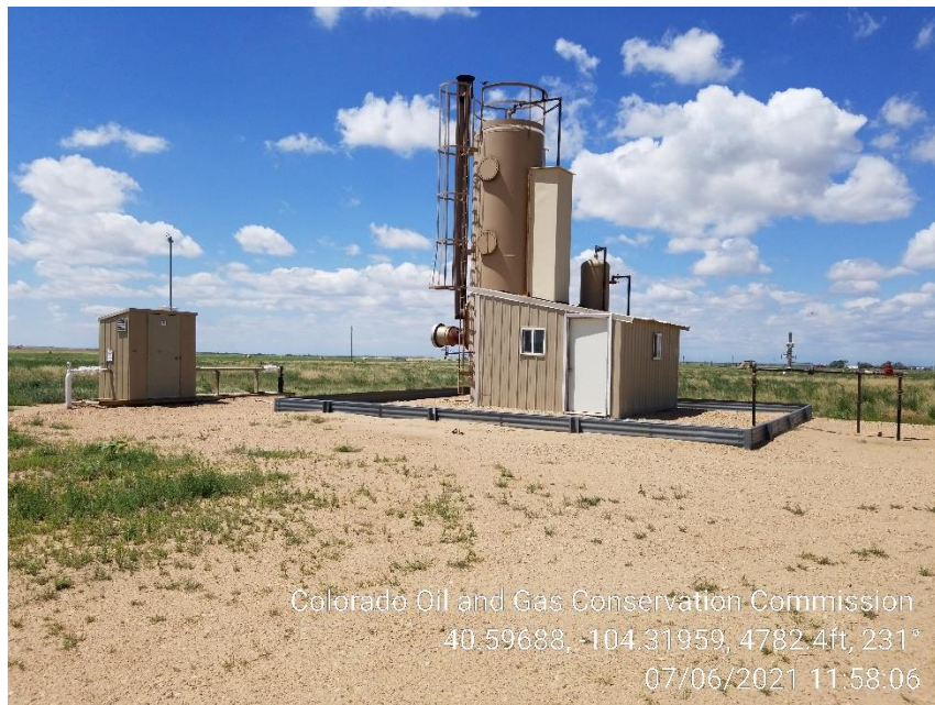
Photo 3 – Heater Treater and Gas Meter
