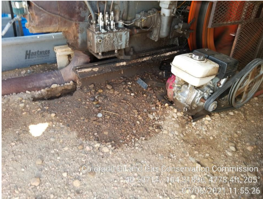
Photo 9 – Stained Soil at Gas Engine
