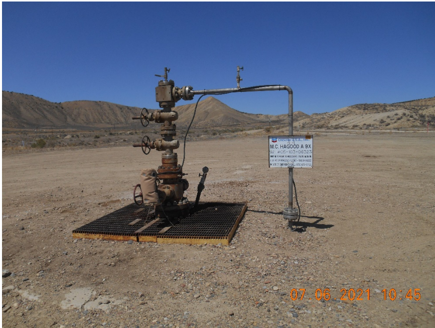
Injection wellhead
