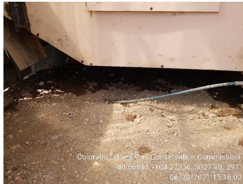
Photo 8 – Stained Soil at Gas Engine
