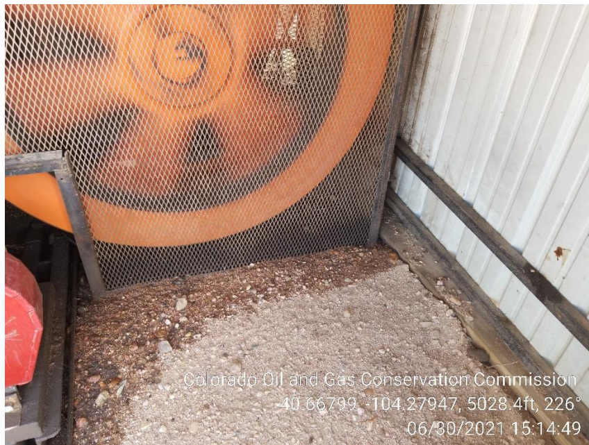
Photo 7 – Stained Soil at Gas Engine
