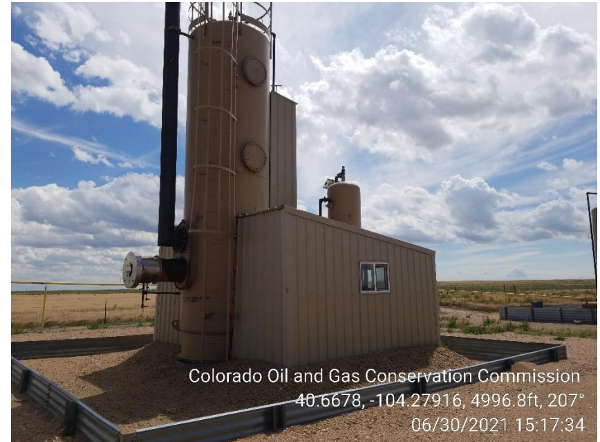
Photo 4 – Heater Treater
