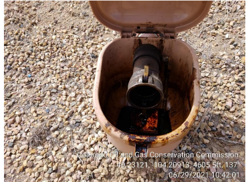
Photo 6 – Loadline Bucket cleaned out
