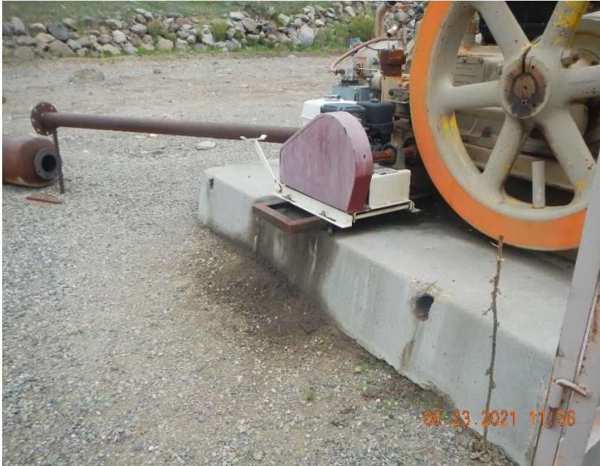
Motor oil stained ground at pump jack motor.
