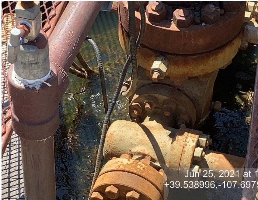
Bubbling around well head
