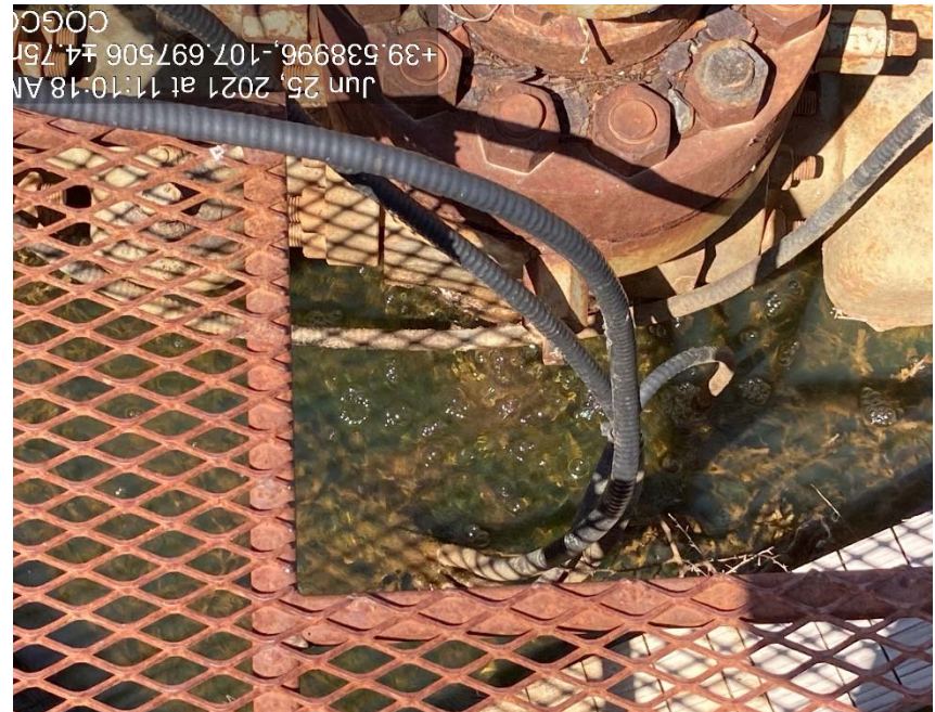
Bubbling around well head
