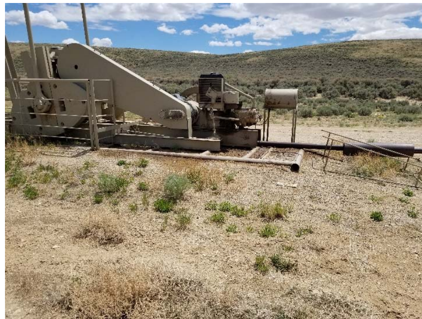
Photo 3. Stained soil at pump jack motor.
