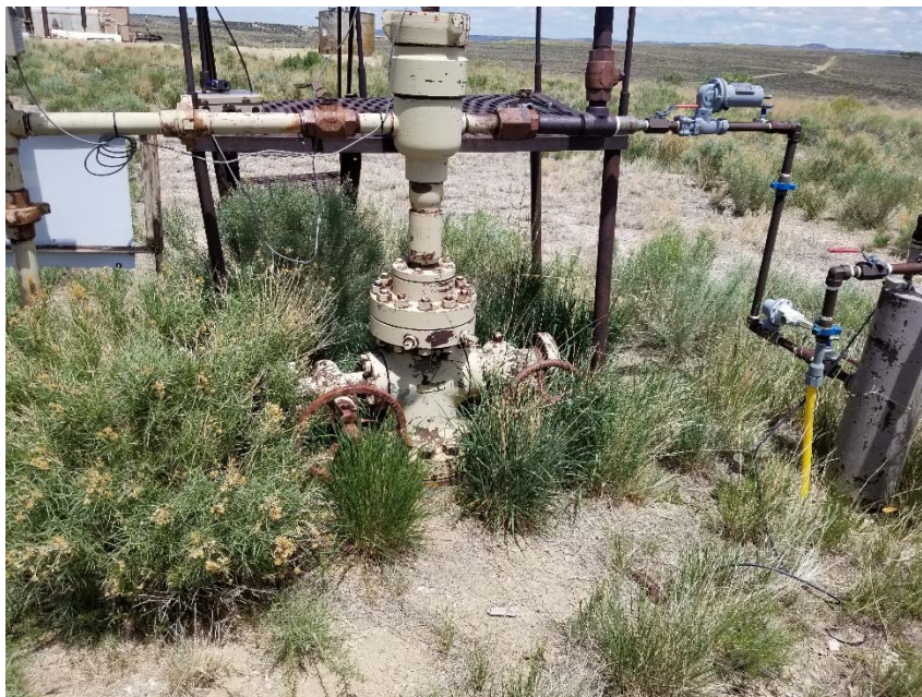
Photo 2. No bradenhead access apparent.
