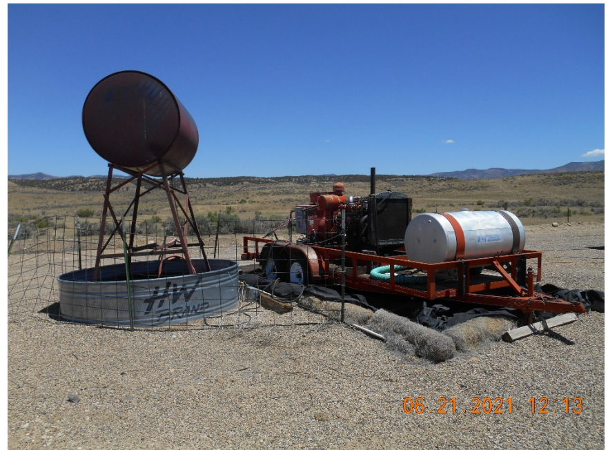
Generator on trailer. Fuel tank with secondary containment
