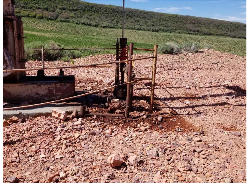
Photo 7. Stained soil at wellhead.
