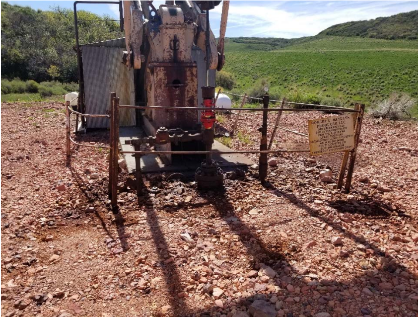
Photo 6. No bradenhead access apparent. Stained soil at wellhead.
