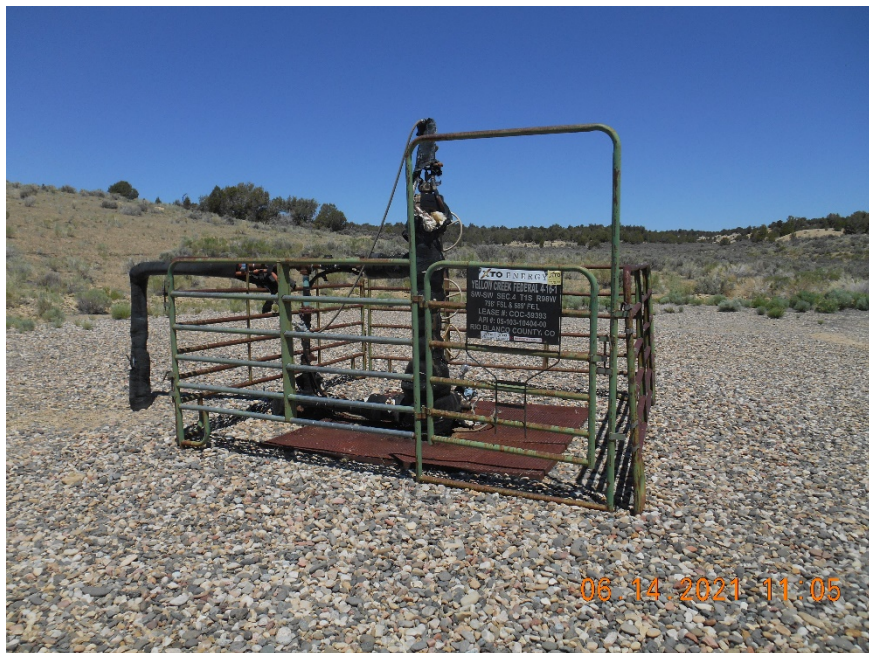
Injection wellhead
