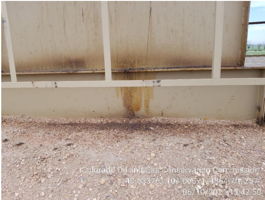
Photo 5 – Stained Soil at Gear Box
