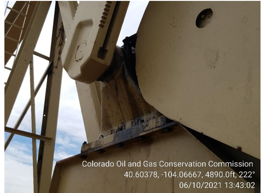
Photo 6 – Gear Box leaking
