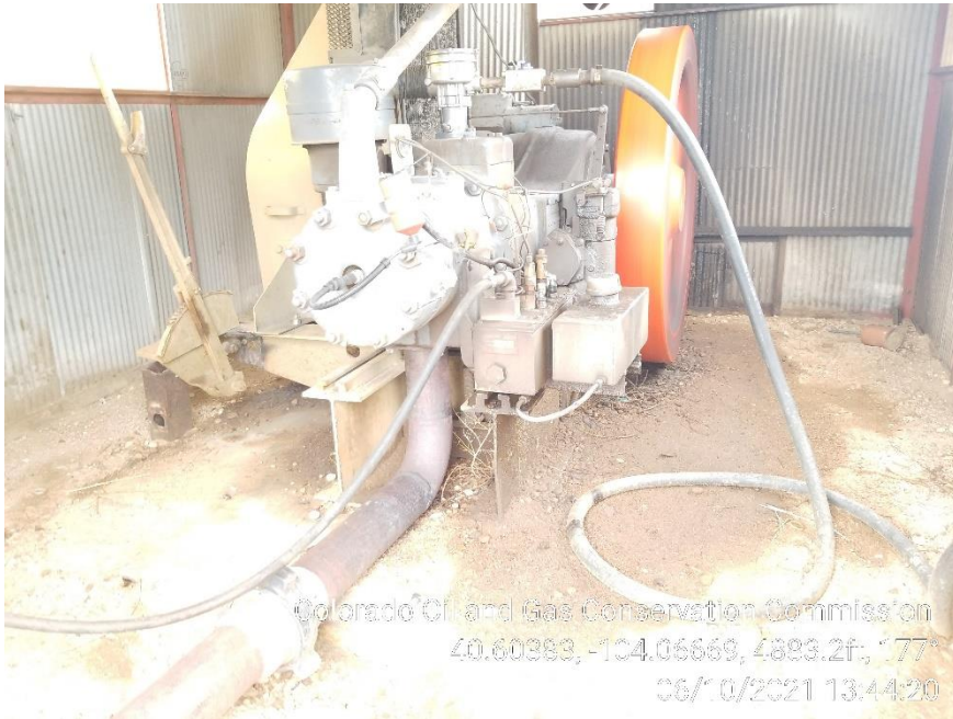
Photo 9 – Stained Soil at Gas Engine
