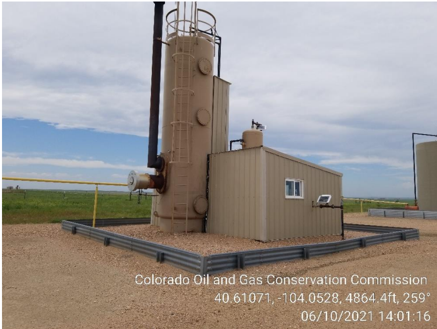
Photo 5 – Heater Treater
