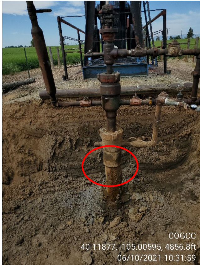
Photo 3 Well casing leak
