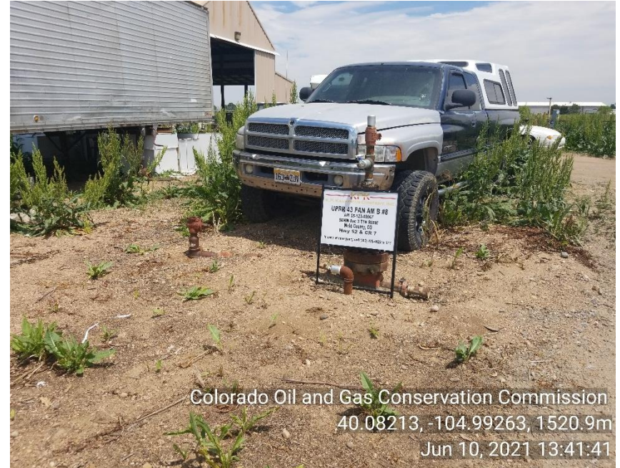
Photo 2 loc pic. Flow line valves not bullplugged and LOTO
