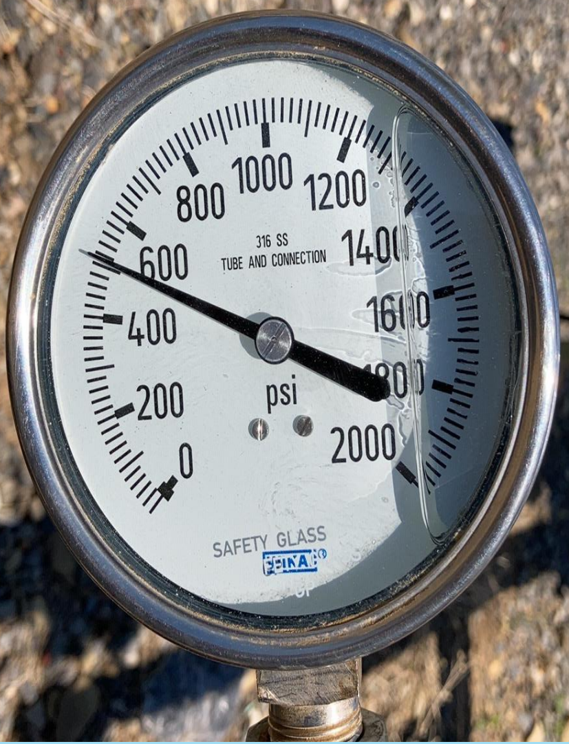
PHOTO 5: 10 MIN. INTO TEST 512 PSI.
