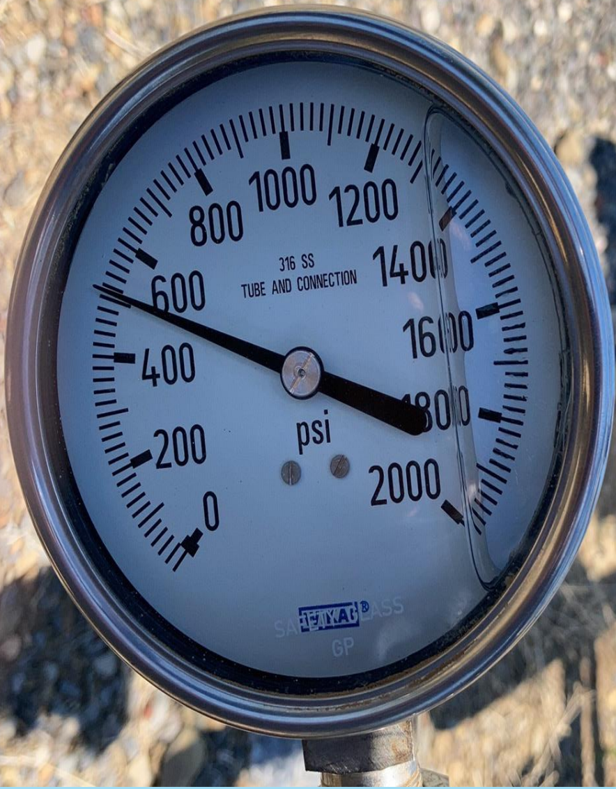
PHOTO 6: 15 MIN. INTO TEST FINAL 511 PSI.
