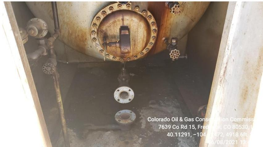
**Photo 9 stained soil inside Horizontal Heated Separator housing**
