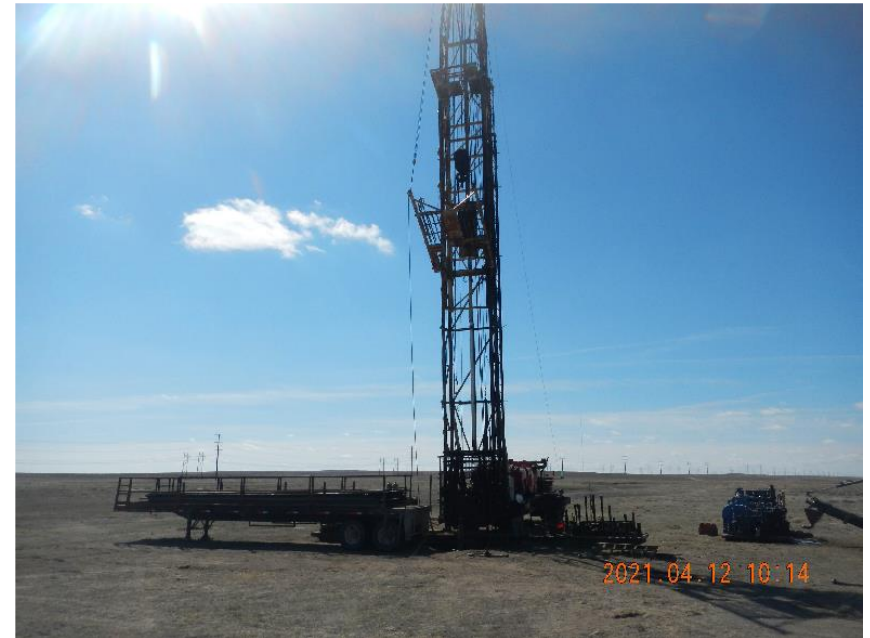
Photo 10: Rig down underway as mast on rig is lowered.
