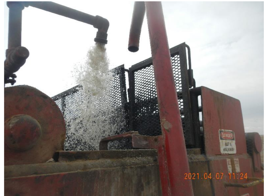
Photo 4: Returns from well to tank during circulation.
