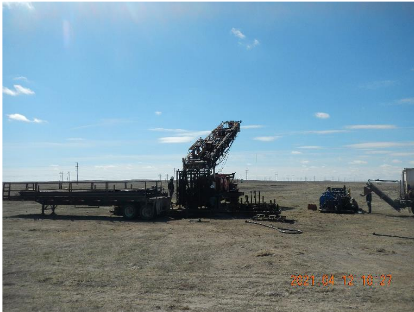
Photo 11: View of mast going into rack as rig down completed.
