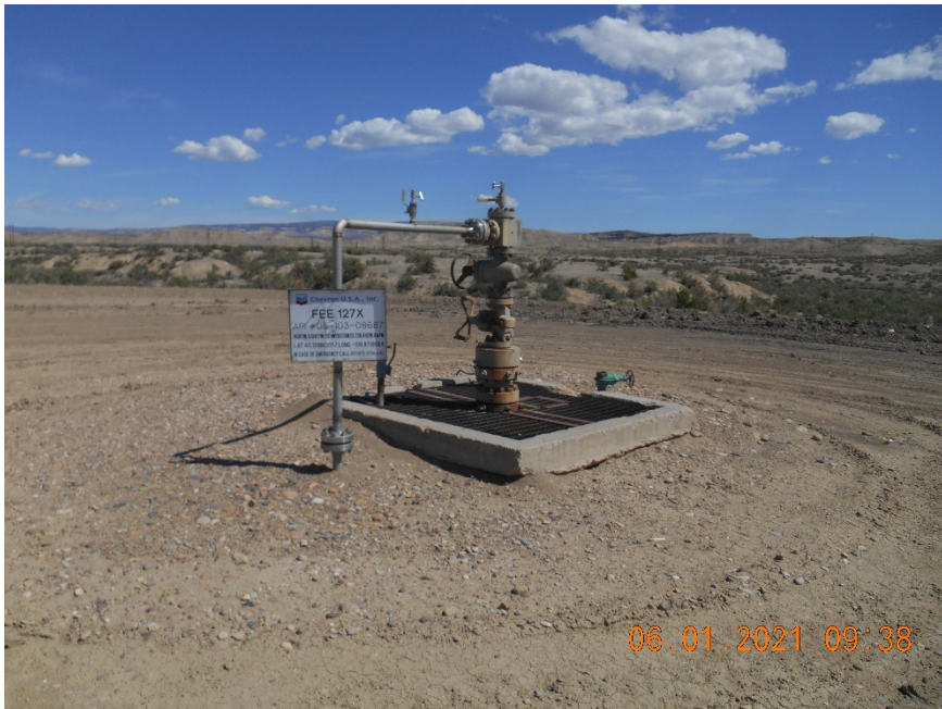
Injection wellhead
