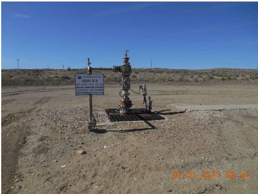
Injection wellhead
