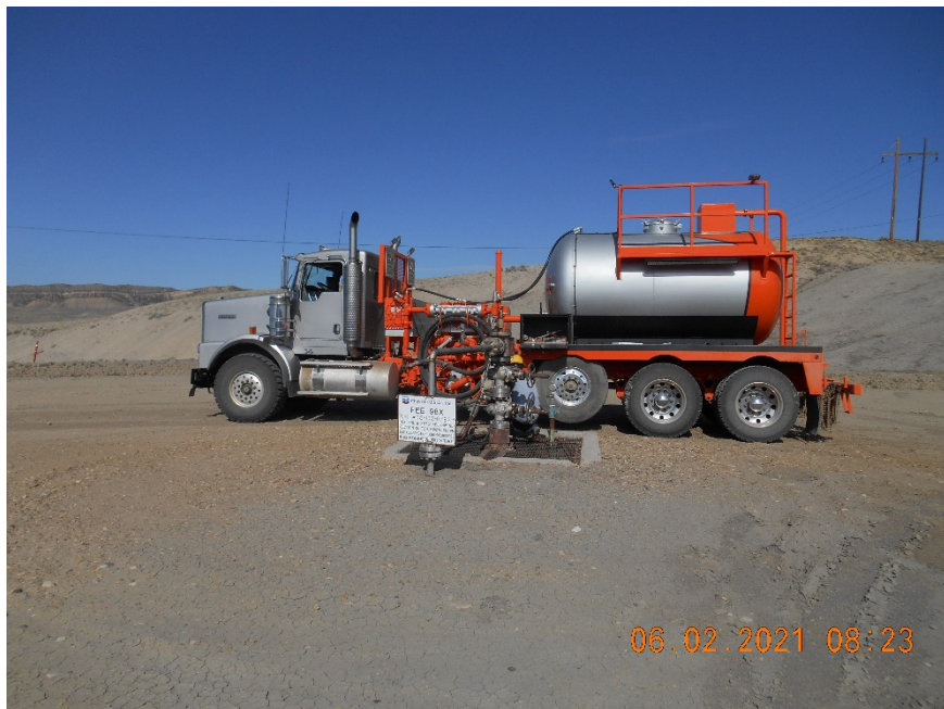
Injection wellhead during MIT.
