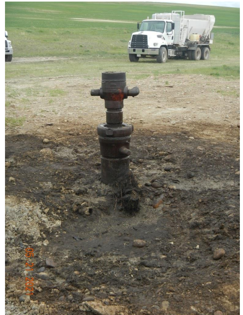
Photo#4: Well head; just completed P&A.
