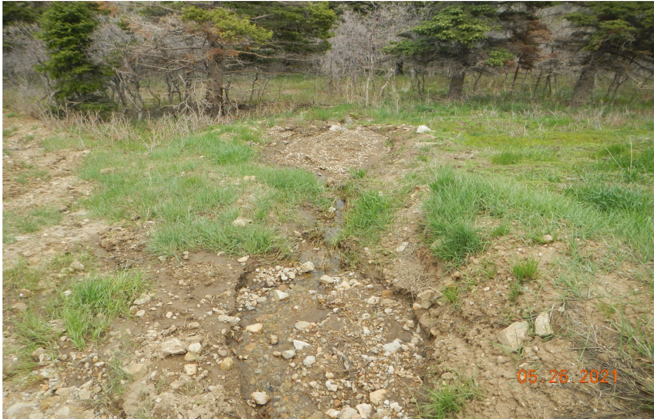
Photo 2. The sediment trap along the road has filled in with sediment.
