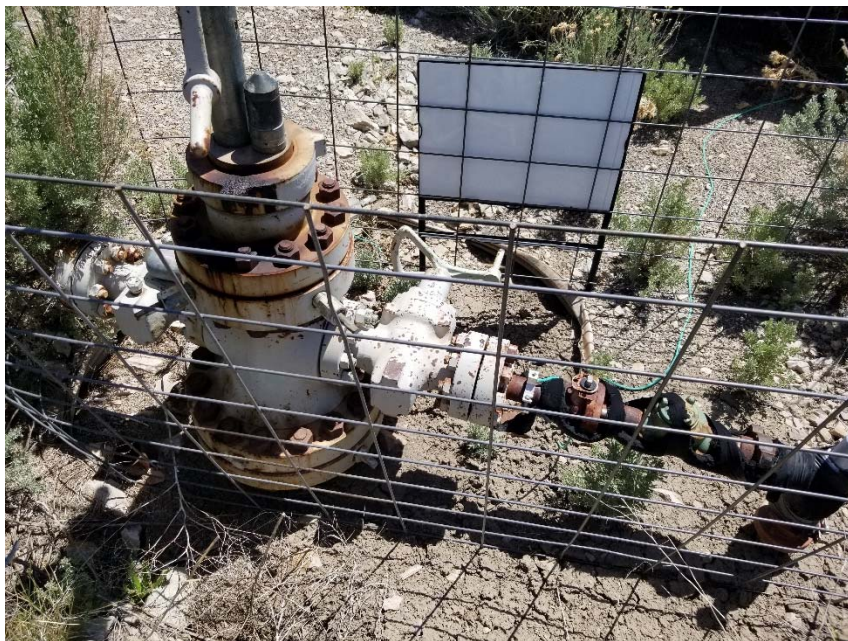
Photo 2. No bradenhead access apparent.
