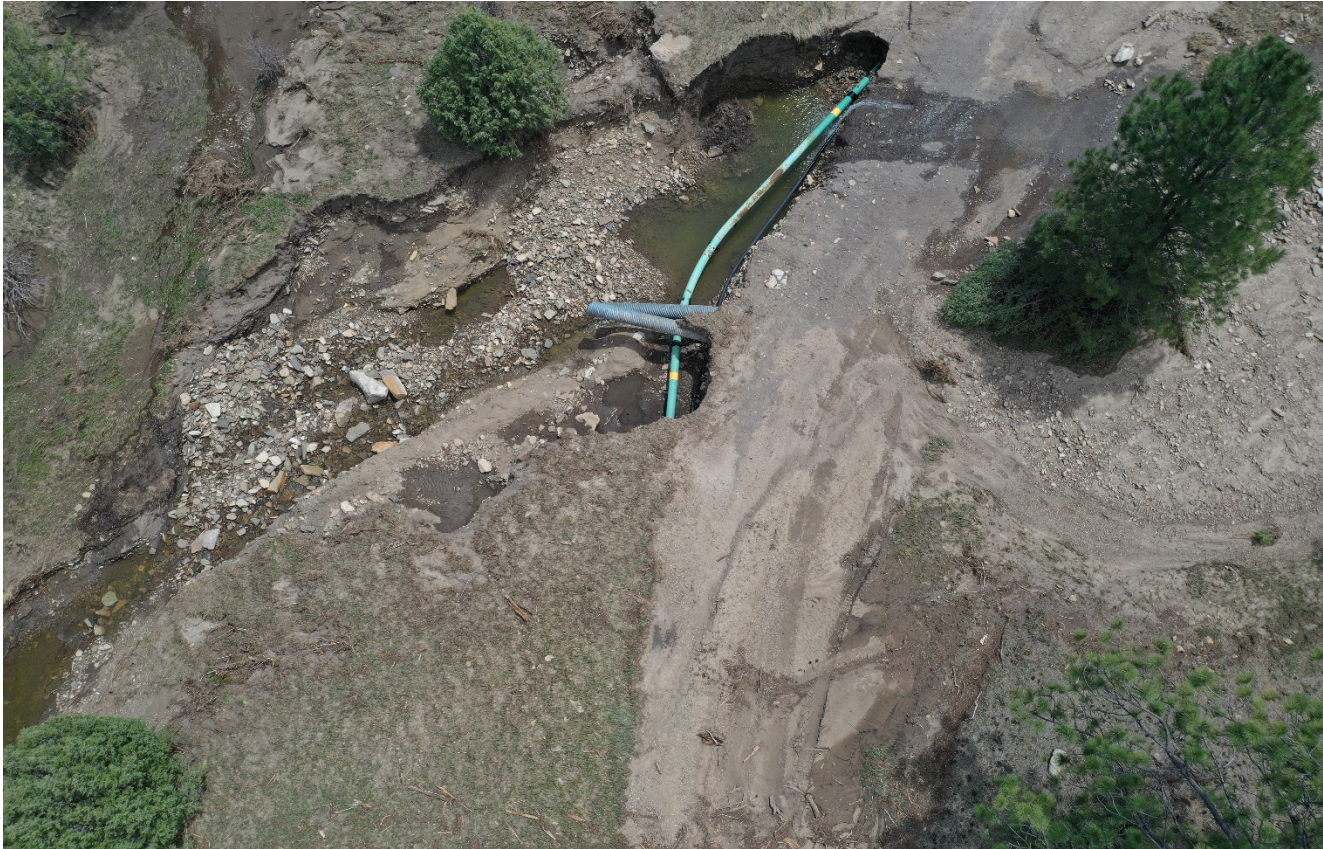
Photo 3. Drone aerial down along the road. Stormwater event has causing significant erosion exposing pipelines.
