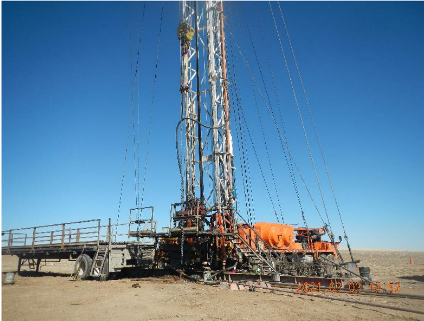
Photo 3: Rig pump and cementing equipment rigged into well pumping squeeze plug.
