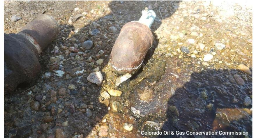
**Photo 5 Bradenhead appears to have a leak from the riser**
