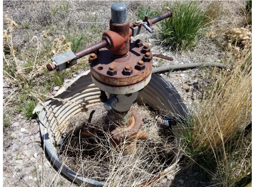
Photo 2. No bradenhead access apparent.
