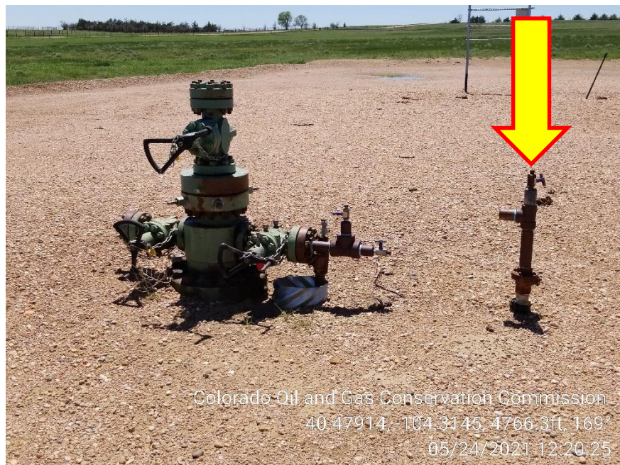
Photo 1 – Wellhead – Unmarked Riser
