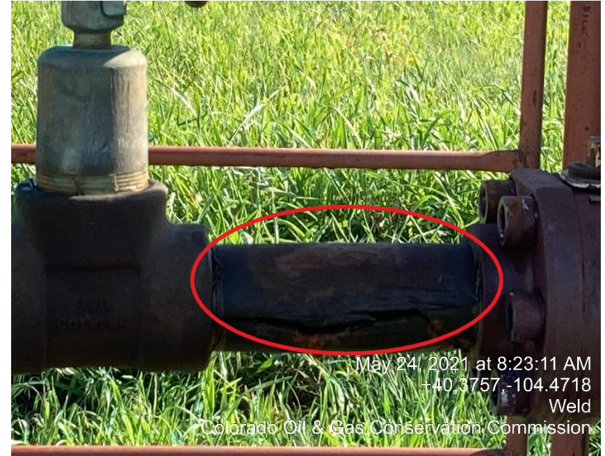
Photo #3 Split tubing on the casing side “mechanical conditions”
