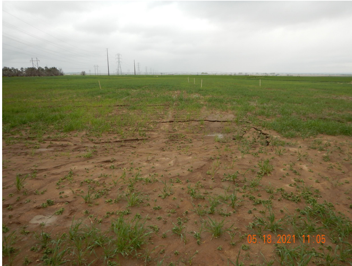
Photo 1. Photo taken from the associated offsite tank battery location, facing South. Photo illustrates subsidence possibly associated with Remediation Project #4185.
