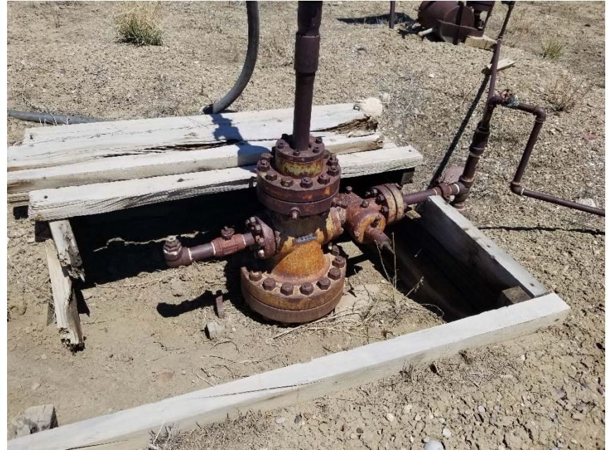
Photo 2. No bradenhead access apparent.
