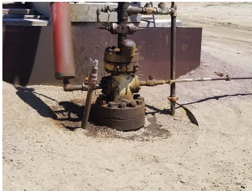
Photo 3. Stained soil at wellhead.
