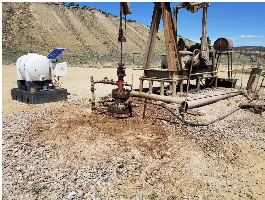
Photo 2. Stained soil around wellhead.
