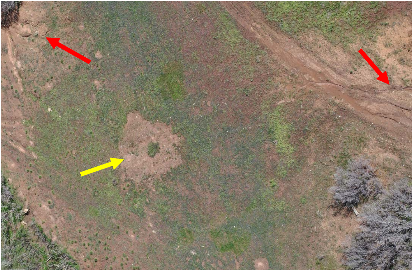
Photo 3. There is erosion evident show at red arrows. The area where tank was location is bare of vegetation growth shown at yellow arrow.
