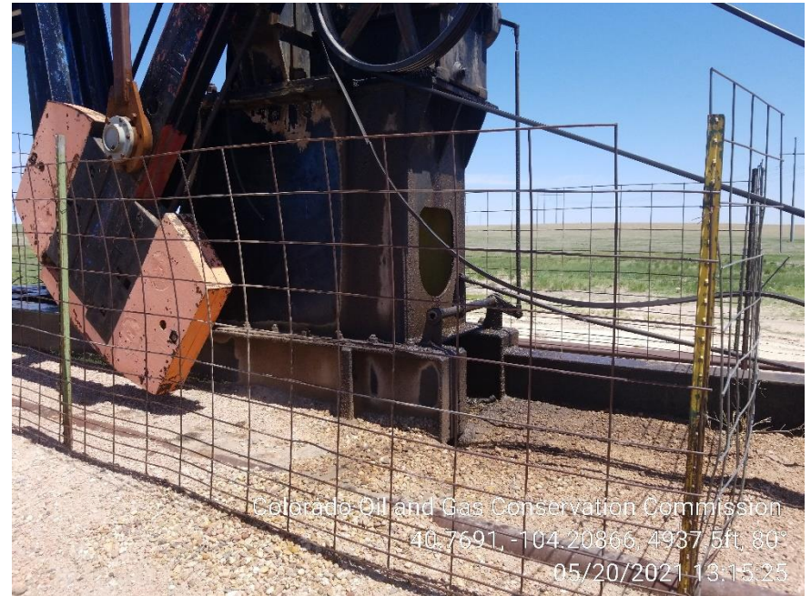
Photo 4 – Gear Box leaking to Soil
