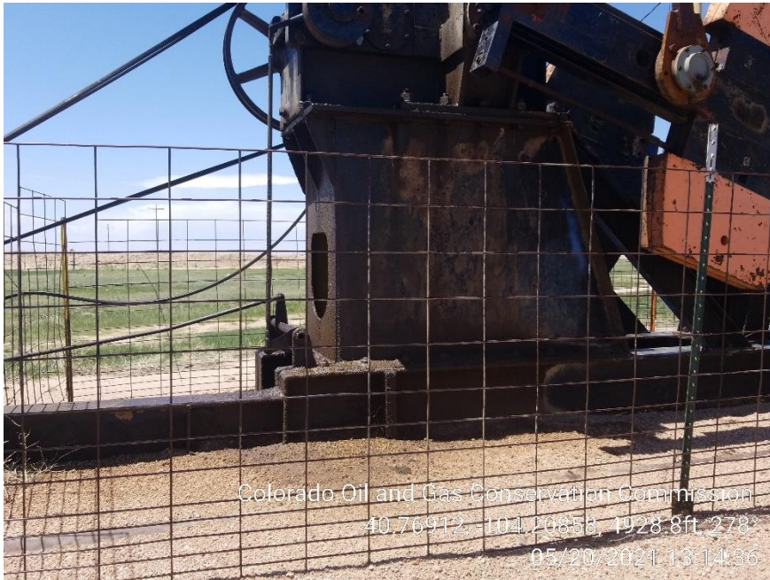
Photo 3 – Gear Box leaking to Soil
