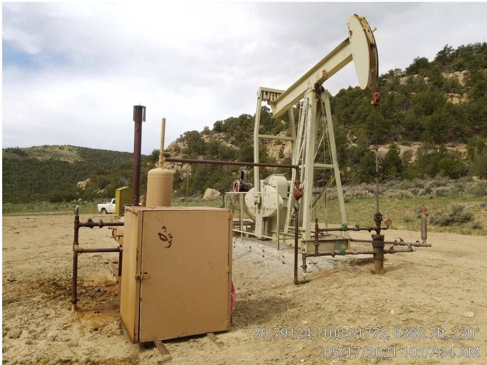
Photo 1. Separator & pump jack.
